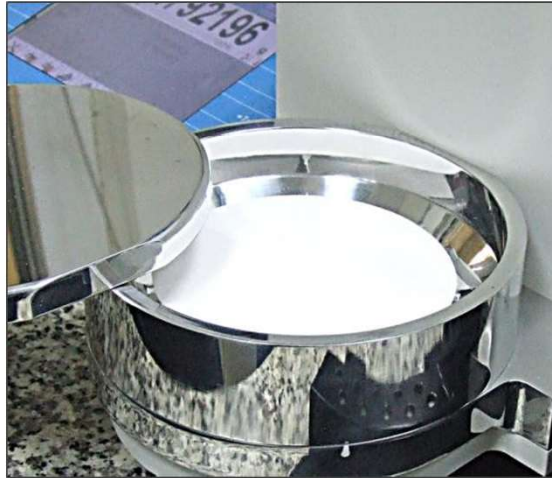
Fig. 14. MYA 5.3Y/F – cellulose filter of 90 mm diameter
