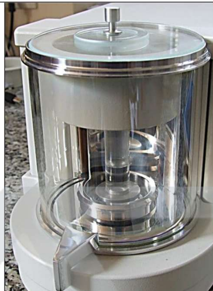
Fig. 32. Weighing liquid by means of so called evaporation ring, designed to check piston pipettes using balance
