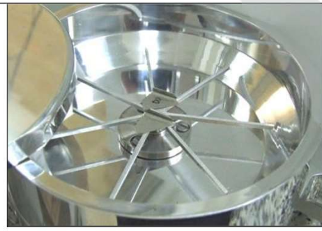
Fig. 24. Balance linearity – testing method 2 linearity points 500 mg ballast weight (B) and 500 mg mass standard
