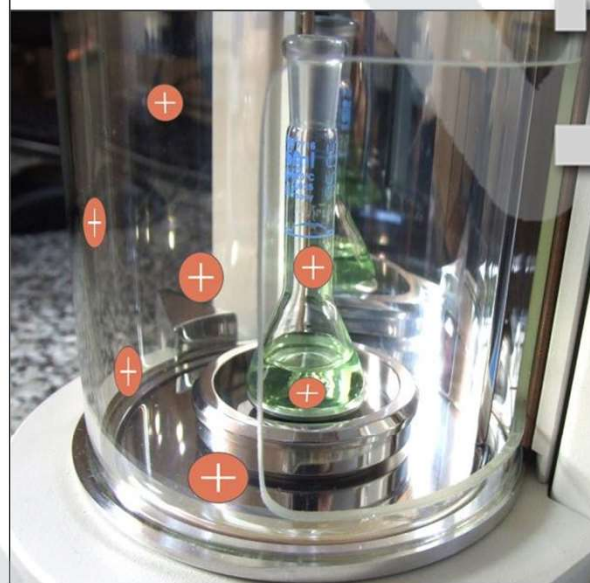
Fig. 16. Unbalanced electrostatic charges
