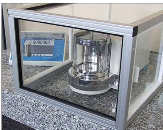
Fig. 15. Microbalance in an anti-draft chamber
