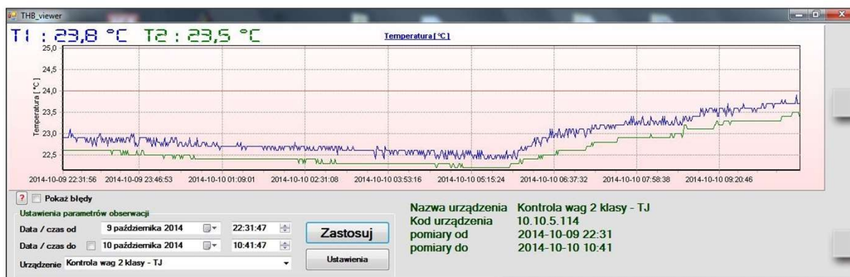
Fig. 8. Diagram of temperature changes occurring within 24-hour-long cycle, easily noticeable temperature growth starting at 6 a.m. is a result of personnel presence
