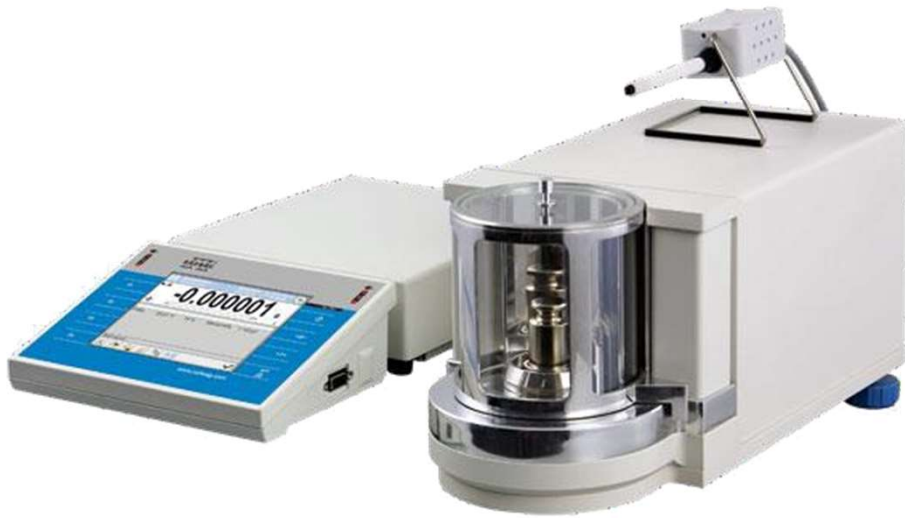
Fig. 29. Microbalance with an external THB sensor
