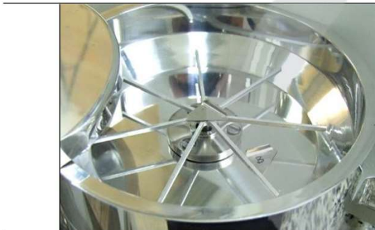
Fig. 23. Balance linearity – testing method 1 linearity point only 500 mg mass standard, (ballast weight is at the bottom of a draft shield)
